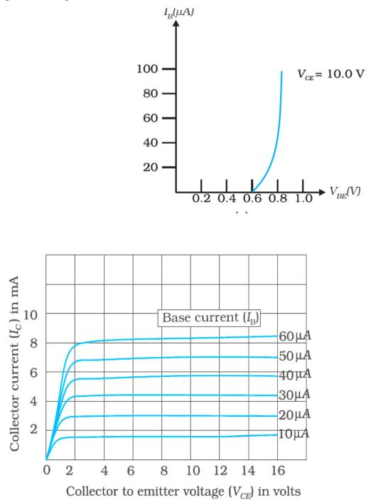
Input and Output Characteristic Curves and Transfer Characteristics
