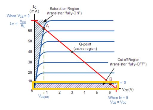
• **Region 3-In Saturation region**, Response is: I<sub>c</sub> = const. V<sub>CE</sub> is constant, being the slope of the curve.
