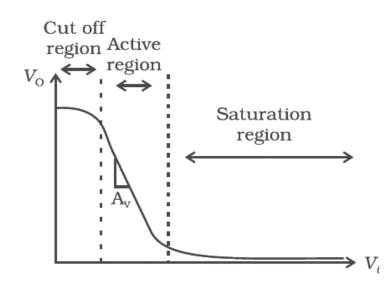
Draw an input ac waveform along the x axis. Note the signal should vary the emitter base forward bias but never make it within the cut off or saturation regions. The variation in  $v_i$  result in variation in  $v_o$ . Observe the output voltage curve to understand phase reversal of  $V_o$  with  $V_i$
