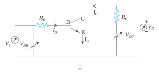
The  $V_{BB}$  supply can be varied from 0V to 5.0 V. The Si transistor has  $\beta_{dc} = 250$  and  $R_{B} = 100$  kW,  $R_{C} = 1$  KW,  $V_{CC} = 5.0$ V. Assume that when the transistor is saturated,  $V_{CE} = 0$ V and  $V_{BE} = 0.8$ V. Calculate
